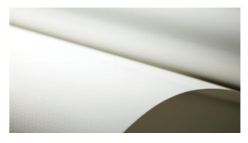
This membrane of type II fulfills all the characteristics required for textile architecture. The low-wick fabric consists of high-strength polyester yarn. Due to the selection of material components it is ensured that our material is low-wick, flame retardant and has permanent fungicidal protection. The weldable surface sealing based on PVDF protects the fabric against any environmental influences.
