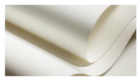
This 700 g/m<sup>2</sup> membrane fulfills all the characteristics required for textile architecture. The low-wick fabric consists of a high-strength polyester yarn type I, offers permanent fungicidal protection and is characterized by its weldable surface sealing based on PVDF. Due to the high strengths, this membrane is used primarily for high-quality halls and tents as wells as for small textile structures. Applications: high-quality halls and tents, textile architecture.
